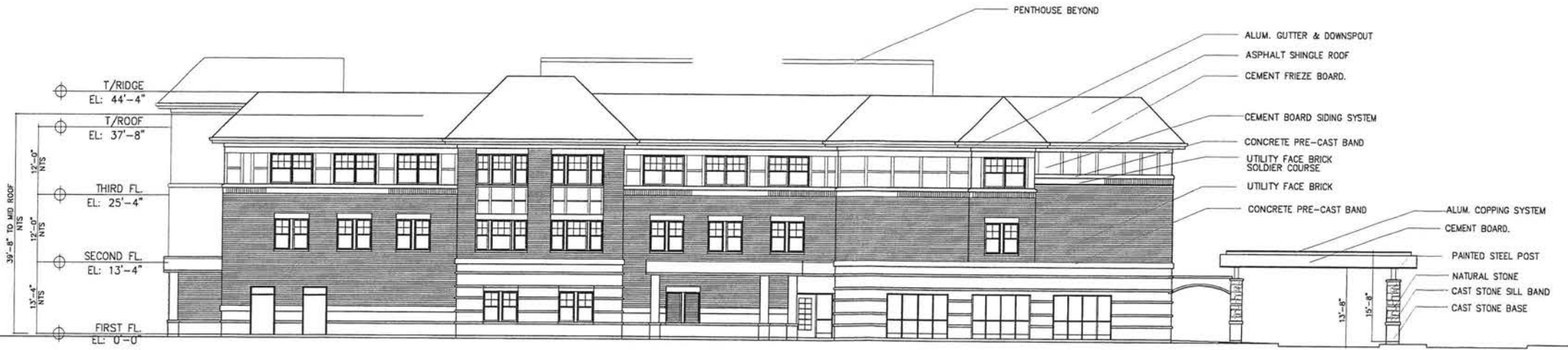
3 EAST ELEVATION SCALE: 3/32"=1'-0"
