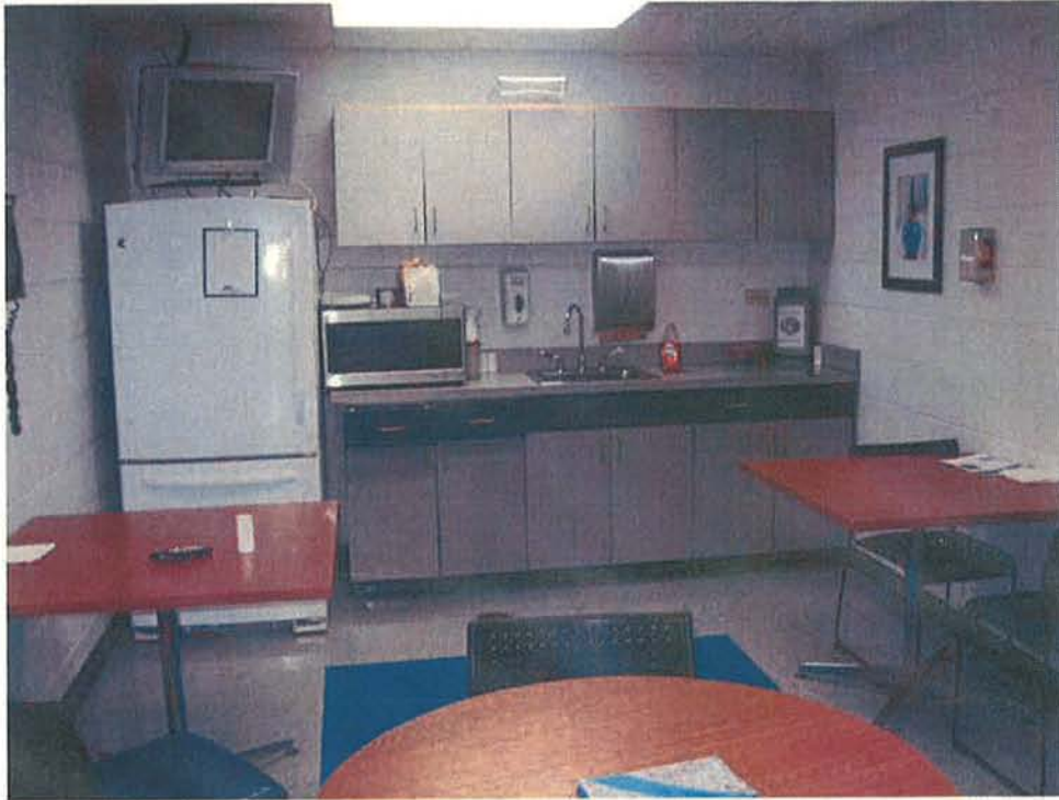
Sinks in common areas require lower countertops and knee space below to adhere to today's accessibility standards.
