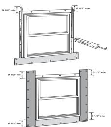
sill flashing long enough to extend a minimum of 9" (229mm) beyond each jamb. Fasten the sill flashing at the bottom and side edges.
