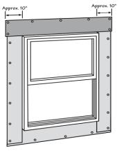
Install rigid head flashing (i.e., drip cap) on top of the top piece of exterior casing, covering trim sheet installed in the previous step. The ends of the rigid head flashing must extend to the outer edges of the exposed legs of the side J-channels. Cut a notch on the ends of the rigid head flashing and bend them down over the sides of the exterior casing. The rigid head flashing must be sealed to the exterior sheathing and to the top of the exterior casing.
