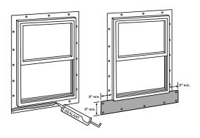
If a nail fin (in new construction) window has been previously installed without flashing, the following instructions should be followed:
