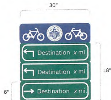
Figure 6: Bicycle Wayfinding design, detailed
