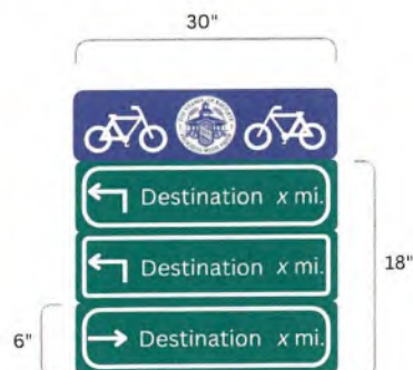
Figure 6: Bicycle Wayfinding design, detailed
