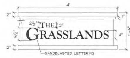
SIGN PANEL DETAILS SCALE: 1"=1'-0"
