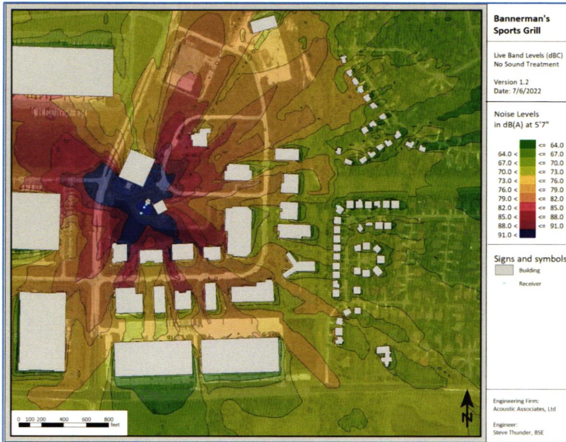
Figure 3 - C-weighted sound contours while a live band is playing on the stage.
