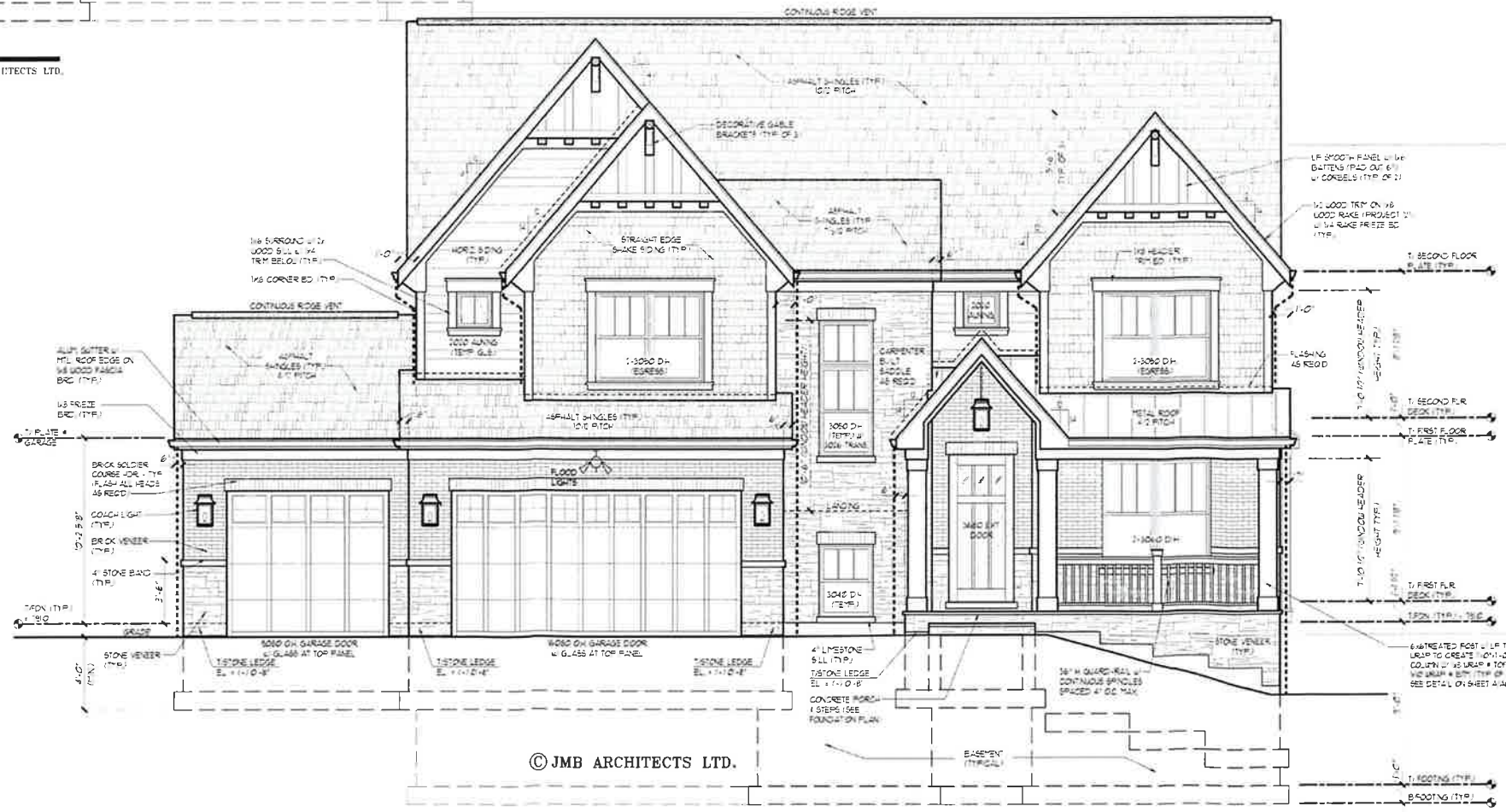
FRONT ELEVATION SCALE 1/4"=1'-0" © JMB ARCHITECTS LTD.
