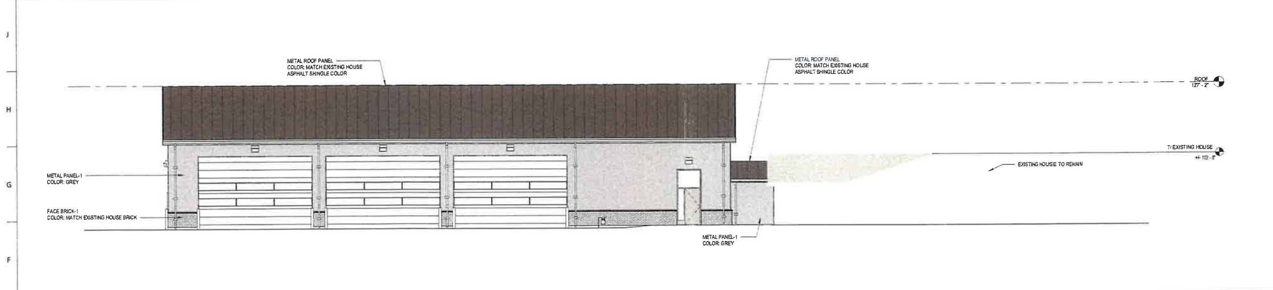
E1 EXTERIOR ELEVATION - NORTH 1/8" = 1'-0"
